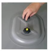
Straighten out the inspection cover, slightly pull it away from the duct wall for precise positioning, and firmly tighten the star knobs.
